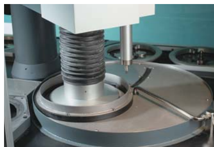
4. Grinding is now in operation. The next specimen holders are ready for collection
