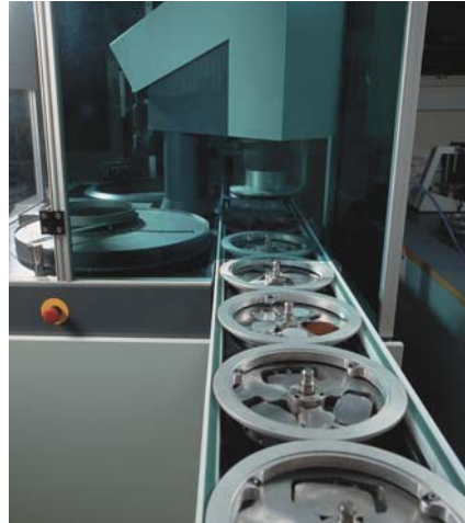
1. Six specimen holders queue up in the conveyer leading into MAPS
