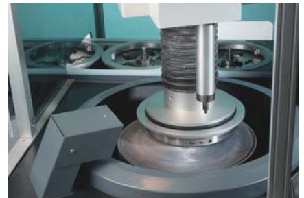
6. After fine grinding the specimen holder moves on to polishing
