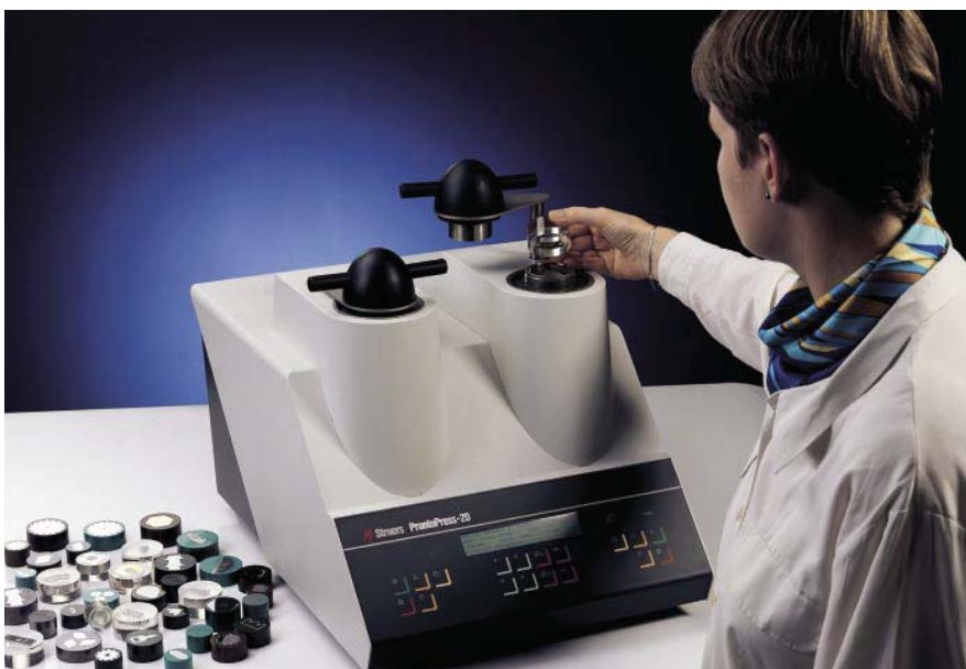
Prontopress-20 with its two cylinders is indispensable when mounting large series of samples in different diameters
