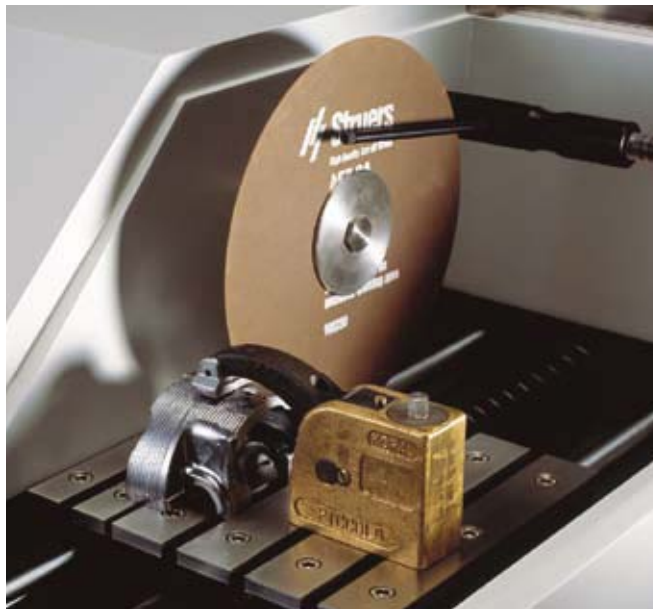
Struers vertical clamping device on the movable cutting table of Secotom-10
