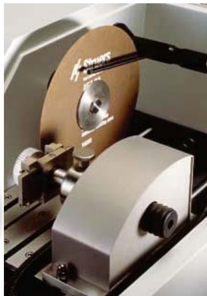
The stand for manual positioning with one of the specimen holders from the Accutom series
