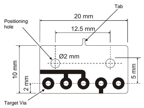
remains connected to the board by a small tab. The tab serves two purposes:
