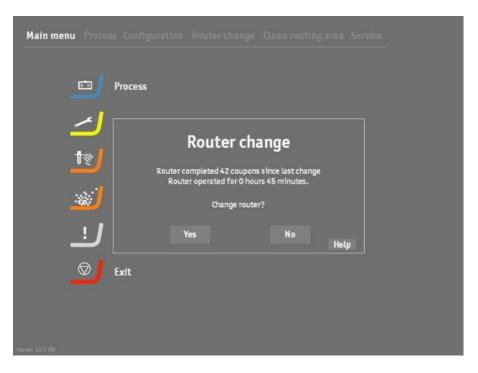
If router change has been confirmed, the safety screen retracts to allow access and the router change instructions are displayed:
