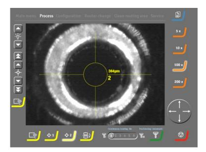
■ Fine position the second target via under the yellow alignment circle by touching the screen at the centre of the target via or by using the table positioning control. An optional adjustment of the diameter of the alignment circle can be done to match the diameter of the target via with the alignment circle diameter buttons.
