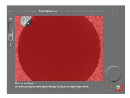
■ Using the mouse, left-click as precisely as possible at one point on the edge of the hole inside the area highlighted in black and white. A new area is highlighted.
