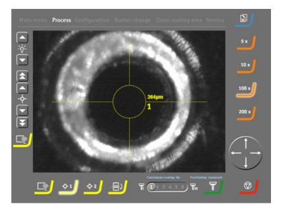
■ Fine position the first target via by touching the screen at the centre of the target via or by using the table positioning control. An optional adjustment of the diameter of the alignment circle can be done to match the diameter of the target via with the alignment circle diameter slider. This makes it easier to align the target via exactly with the alignment circle.
