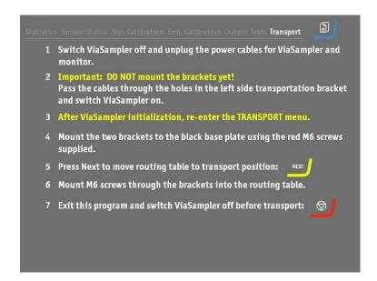
Mount the two brackets to the black base plate using the red M6 screws supplied.
