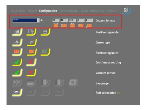
The possible coupon size largest is approximately 45 x 45 mm or 5 x 50 mm, depending on the angle of the coupon in relation to the routing well, which sets the physical limits.
