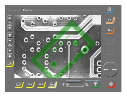
In the screen capture above, a via will interfere with the drilling of the left side positioning hole, so the area to be routed should be flipped around the line of targets to avoid this, as illustrated in the next screen shot:
