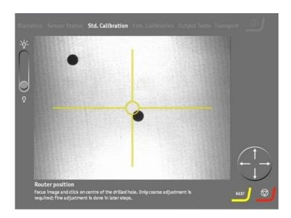
At this stage, it is necessary to make a coarse correction of the camera alignment. Click at the centre of the drilled hole, so that the hole moves to the centre of the yellow circle.
