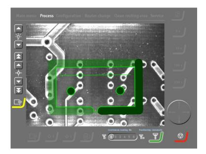
When routing is complete, the display reverts to a live camera view of the board. It is now possible to begin the coupon production process again, to route additional coupons from the board.
