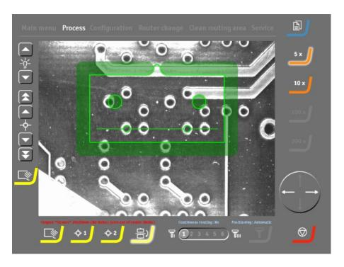
If a large coupon is tilted at an angle that will result in a conflict with the edges of the routing well, then the routing process cannot be started.
