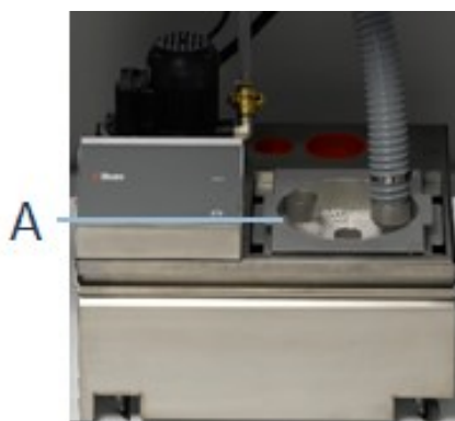
A Static filter unit
