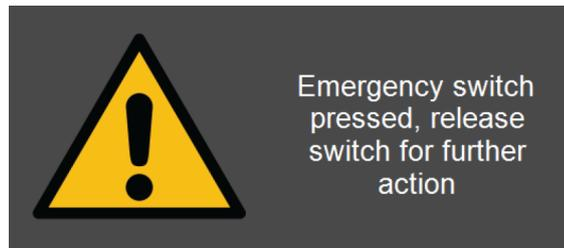
If the emergency stop is activated during start-up, an error message is shown.
