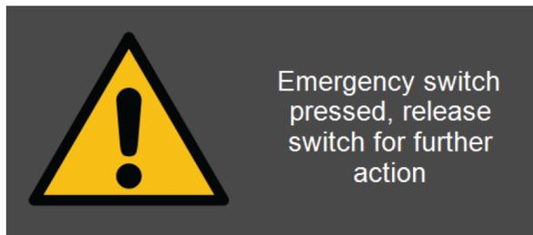
The machine stops and a message is shown prompting you to release the emergency stop. If this does not happen, contact Struers Service.
