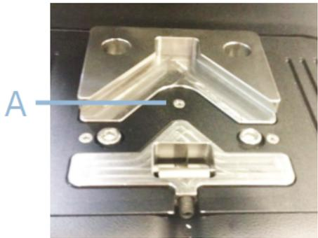
5. Tighten the fixation screw to secure the stage in place. [A]
